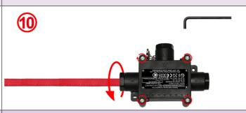
10: Slide the flat cable gasket into the cable gland and tighten the nut. Max. tightening torque 3N.m. If not yet made connect the other cable and close the lid.
