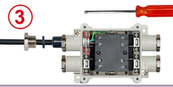
$\bf 3$  : Put the saddle and its 2 screws on the cable and tighten the screws. Recommanded torque for the 3 screws 1.6 Nm.
