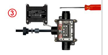
**3**: Put the saddle and its 2 screws on the cable and tighten the screws. Recommanded torque for the 2 screws **1**.6 Nm.
