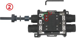
1: Remove outer jacket on 24mm. Then strip the conductors on 10mm. Eventually, crimp cable shoes. Slide the cable gland nut on the cable. Select the compatible diameter gasket and slide it too on the cable.
