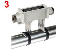
3: Secure the plate and its legs to the tube with metal clamps (recommended), or if necessary, nylon ties. Screw the 2 legs on the bracket A and enclosure sub-assembly
