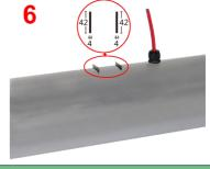
6: If the thermal insulation has a metal protective sheath, make two straight incisions of 4×42mm at a distance of 52mm to allow each of the two legs to pass. Provide the orifice(s) to exit the cables from the metal protection. Equip them with M25 cable glands with the appropriate gaskets for the dimensions of the cables. Close the metal sheath around the tube. Wrap insulation on the pipe, just making two straight cuts for the legs
