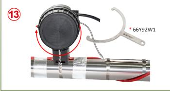
13: Connect the conductors according to the wiring diagram. Connect the power supply cable. Close the control box.
