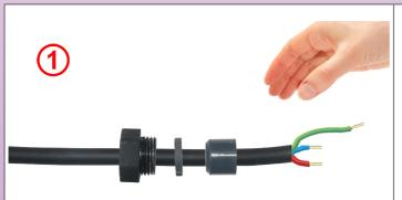
1: Unsheath the cable according to the plan above then cut the conductors as required and strip them to 10mm. Eventually, crimp cable shoes.
