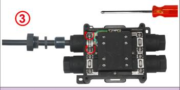
**3:** Slide the ground wire under the ground terminal square washer and tigthen the screw. Recommanded torque 1.6 Nm.
