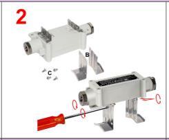
2: Assemble the two feet with the four screws. Take the 2 legs (B) and the 4 screws (C)
