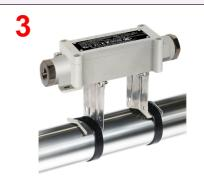
3: Secure the plate and its legs to the tube with metal clamps (recommended), or if necessary, nylon ties. Screw the 2 legs on the bracket A and enclosure sub-assembly
