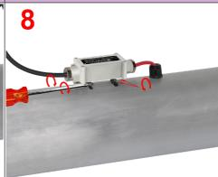
8: Refit the ends of the legs with the 4 screws on the box.
